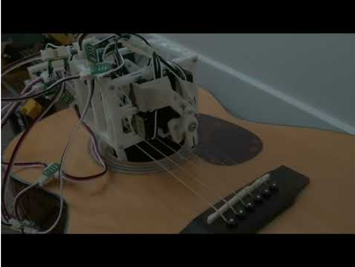
Figure 9: MegCell Strumming Arm Mechanism https://www.youtube.com/watch?v=MpRi8xJrh24
